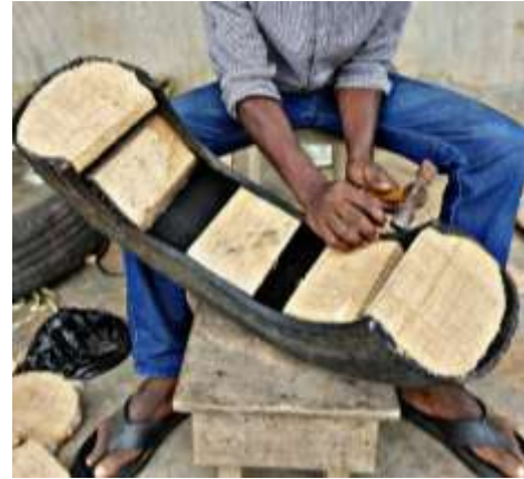
Plate 8: Cutting of tyres into two to create a back rest Plate 9: Insertion of plywood pieces into
