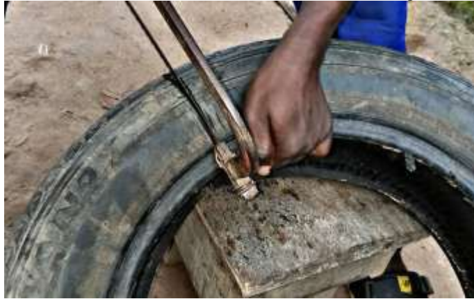
Plate 8: Cutting of tyres into two to create a back rest Plate 9: Insertion of plywood pieces into
