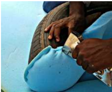
Plate 4: Affixing foam to the tyre with gun stapler
