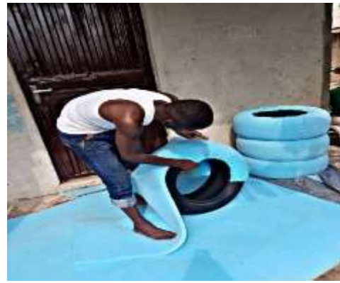
Plate 3: wrapping of foam on the tyres
